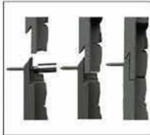
9. Upper panel interlocks with lower panel, screws are invisible
